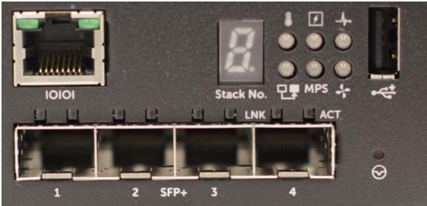
Figure 1-3. Dell Networking N1524P Close-up
